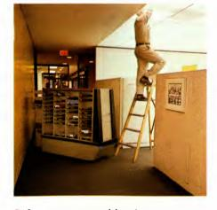
Soft, pressure-sensitive bumpers automatically stop Mailmobile when obstacles are in its path. Travel is halted until obstacle is removed, then resumes automatically. A non-contact obstacle detection system is available as an option.
